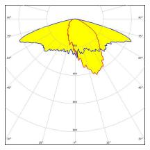
IESNA Type II (medium) beam, applicable for European P-class standard pedestrian lighting and M-class roads
