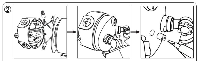
3) To paste the EVA Gasket onto the surface of Junction Box.
