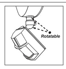
6) To adjust the sensor device and to set the head of lamp to suitable position.
